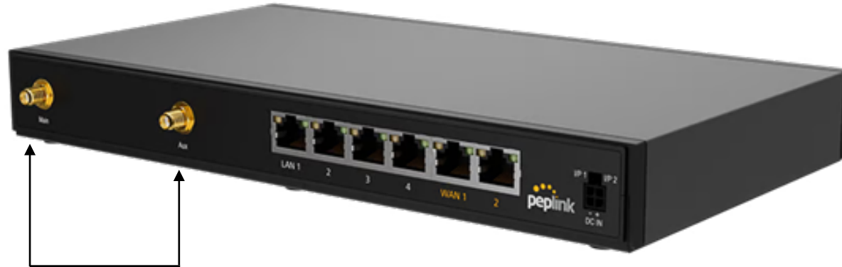
Cellular Ports Antenna Connector Ends SMA Male
